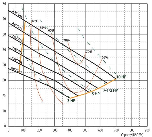
The curves reflect maximum performance characteristics without exceeding full load. Operation is recommended in the bounded area with operational point within the curve limit. Performance curves are based on actual tests with clear water at 70° F and 1280 feet site elevation.
