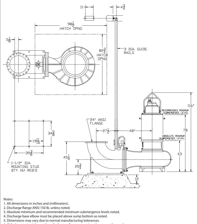
6. If discharge pipe is larger than discharge elbow, eccentric reducer must be used limited to 2X larger maximum.
