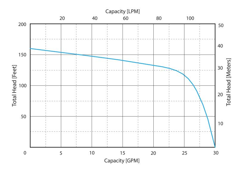
The curves reflect maximum performance characteristics without exceeding full load. Operation is recommended in the bounded area with operational point within the curve limit. Performance curves are based on actual tests with clear water at 70° F and 1280 feet site elevation.
