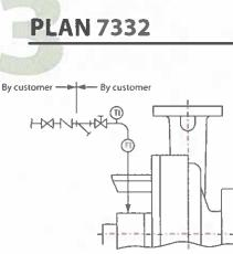
Injection in the mechanical seal from a source of clean fluid.
