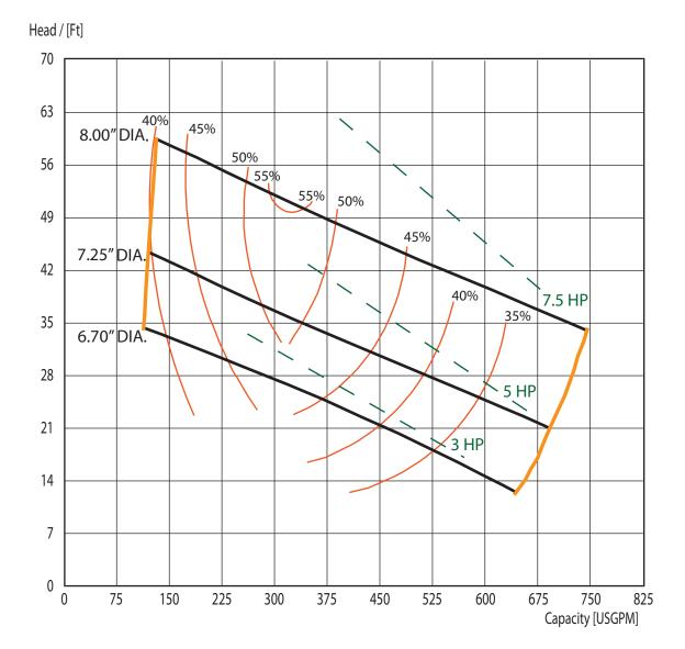
The curves reflect maximum performance characteristics without exceeding full load. Operation is recommended in the bounded area with operational point within the curve limit. Performance curves are based on actual tests with clear water at 70° F and 1280 feet site elevation.
