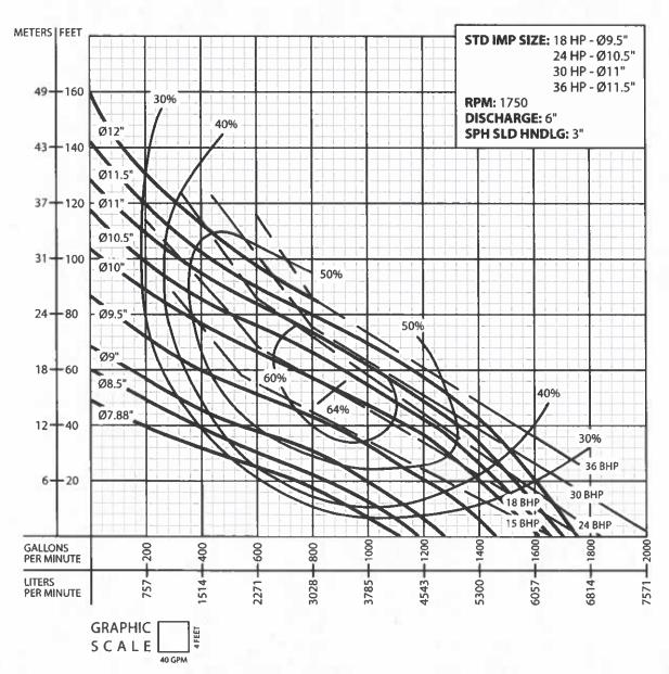
Testing is performed with water specific gravity of 1.0 @ 68 °F (20 °C); other fluids may vary performance.
