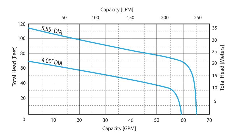
The curves reflect maximum performance characteristics without exceeding full load. Operation is recommended in the bounded area with operational point within the curve limit. Performance curves are based on actual tests with clear water at 70° F and 1280 feet site elevation.
