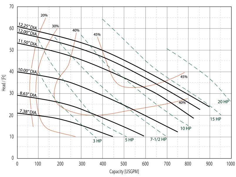
The curves reflect maximum performance characteristics without exceeding full load. Operation is recommended in the bounded area with operational point within the curve limit. Performance curves are based on actual tests with clear water at 70° F and 1280 feet site elevation.
