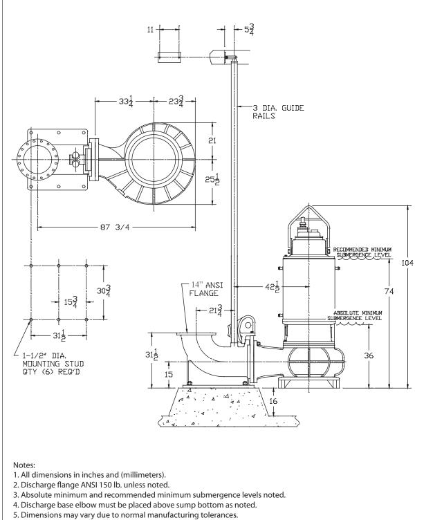
6. If discharge pipe is larger than discharge elbow, eccentric reducer must be used limited to 2X larger maximum.
