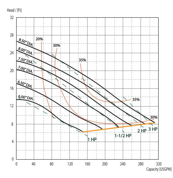
The curves reflect maximum performance characteristics without exceeding full load. Operation is recommended in the bounded area with operational point within the curve limit. Performance curves are based on actual tests with clear water at 70° F and 1280 feet site elevation.
