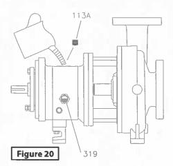
The gland should be tightened evenly to achieve a good seal, excessive tightening of the gland can cause premature wear on the packaging and/or sleeve.
