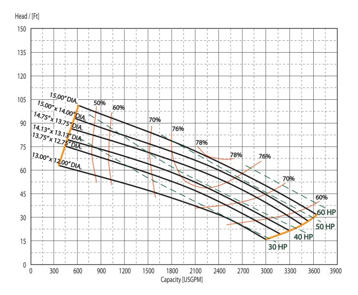
The curves reflect maximum performance characteristics without exceeding full load. Operation is recommended in the bounded area with operational point within the curve limit. Performance curves are based on actual tests with clear water at 70° F and 1280 feet site elevation.
