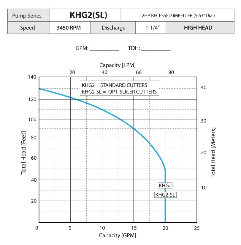
The curves reflect maximum performance characteristics without exceeding full load. Operation is recommended in the bounded area with operational point within the curve limit. Performance curves are based on actual tests with clear water at 70° F and 1280 feet site elevation.
