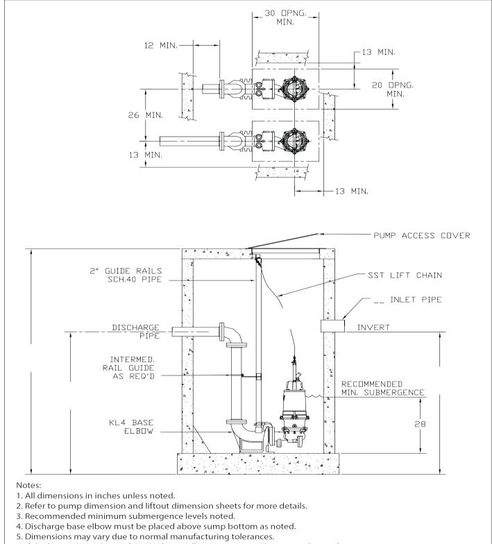
6. If discharge pipe is larger than discharge elbow, eccentric reducer must be used limited to 2X larger maximum.
