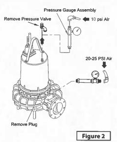
Pressure builds up extremely fast, increase pressure by "TAPPING" air nozzle. Too much pressure will damage seal. DO NOT exceed 10 PSI in housing and 20-25 PSI in seal chamber.
