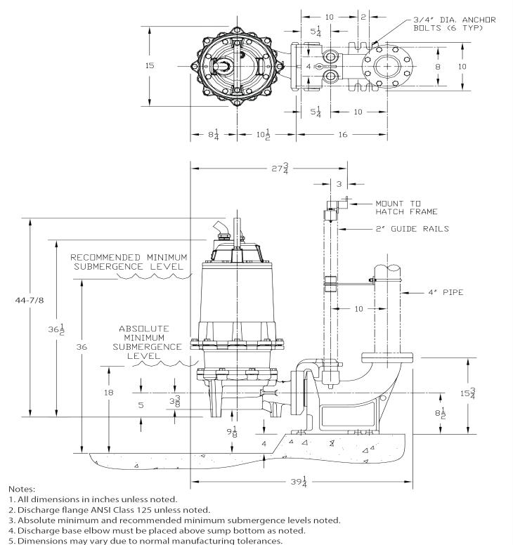
6. If discharge pipe is larger than discharge elbow, eccentric reducer must be used limited to 2X larger maximum.
