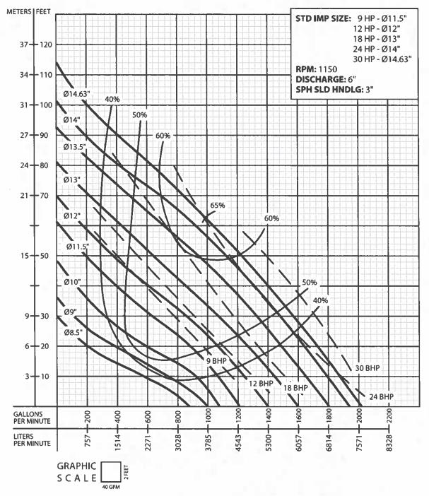
Testing is performed with water specific gravity of 1.0 @ 68 °F (20 °C); other fluids may vary performance.
