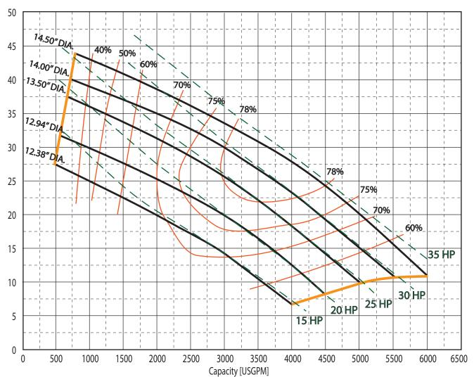
The curves reflect maximum performance characteristics without exceeding full load. Operation is recommended in the bounded area with operational point within the curve limit. Performance curves are based on actual tests with clear water at 70° F and 1280 feet site elevation.
