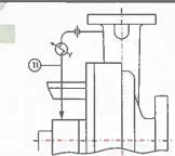
Recirculation of the volute to the heat exchanger and then to the mechanical seal flange.
