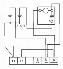
SINGLE PHASE 230 VOLT AC Capacitor/Relay Pack For Control Panels SINGLE-PHASE 230V AC
