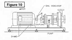
Horizontal: Consist of installing a dial indicator (see Figure 11) in the top half of the coupling "X", leaving it fixed, and then proceeds to inspect the four cardinal points of the "Y" coupling. If readings exceed 0.002" (0.05 mm), means that the motor is offset from the top down, so install or remove equal amounts of shims at the motor feet, to correct the readings.
