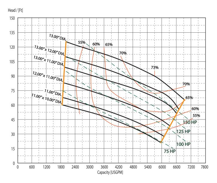
The curves reflect maximum performance characteristics without exceeding full load. Operation is recommended in the bounded area with operational point within the curve limit. Performance curves are based on actual tests with clear water at 70° F and 1280 feet site elevation.
