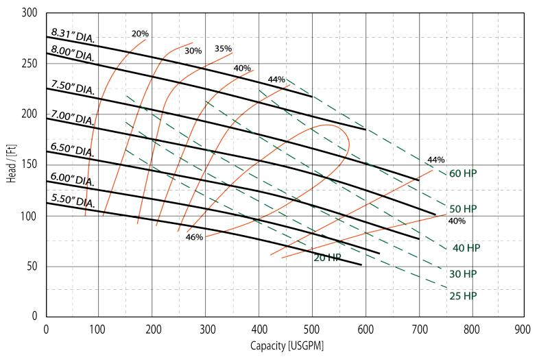
The curves reflect maximum performance characteristics without exceeding full load. Operation is recommended in the bounded area with operational point within the curve limit. Performance curves are based on actual tests with clear water at 70° F and 1280 feet site elevation.
