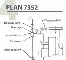
¥ External fluid container without pressurizing; forced circulation.
